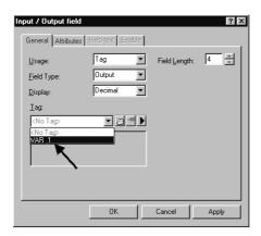
Set up a data area for the tag in the PLC. Using the input field, it is possible to enter a process value in the PLC which is then issued via the output field.
