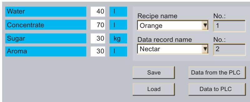
In the recipe screen, the values are saved in recipe tags. Depending on the configuration, the recipe values are transferred between the PLC and the HMI device either immediately or after the respective operating element has been activated.
