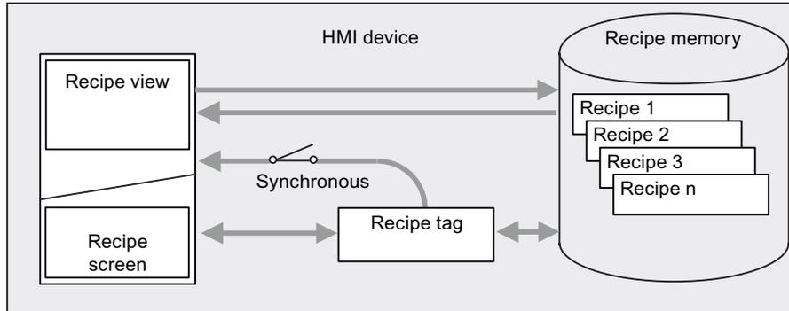
Complete recipe data records are loaded from or saved to the recipe memory on the HMI device in the recipe view.
